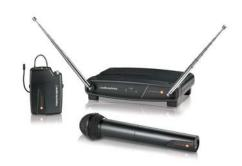
user-adjustable squelch; rugged unidirectional dynamic element on the handheld microphone/transmitter; variable microphone trim control and multi-color battery/power indicator (with AA operation on transmitters); and a professional locking connector on the UniPak body-pack transmitter.
